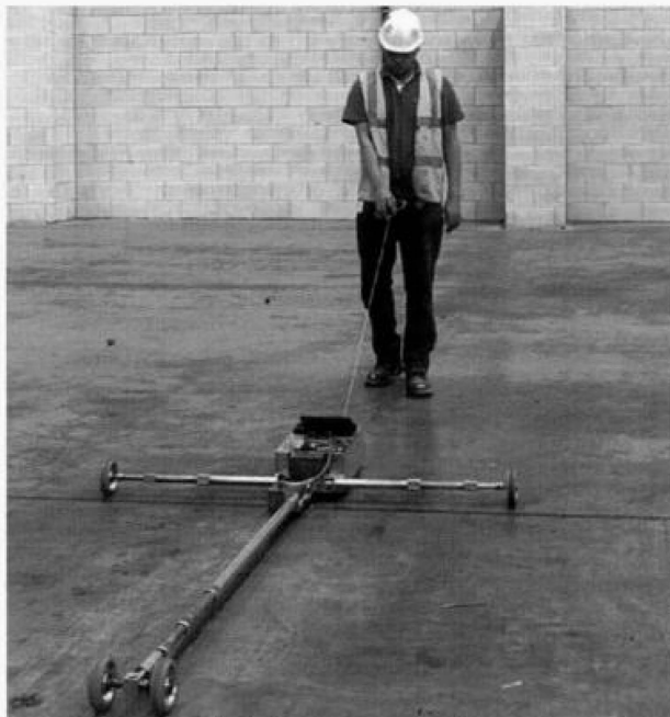
Figure C2: Surveying a defined-movement area with a profilegraph prior to installation of racking
